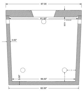
Tank joint sealed with CS 101 butyl rubber sealant
